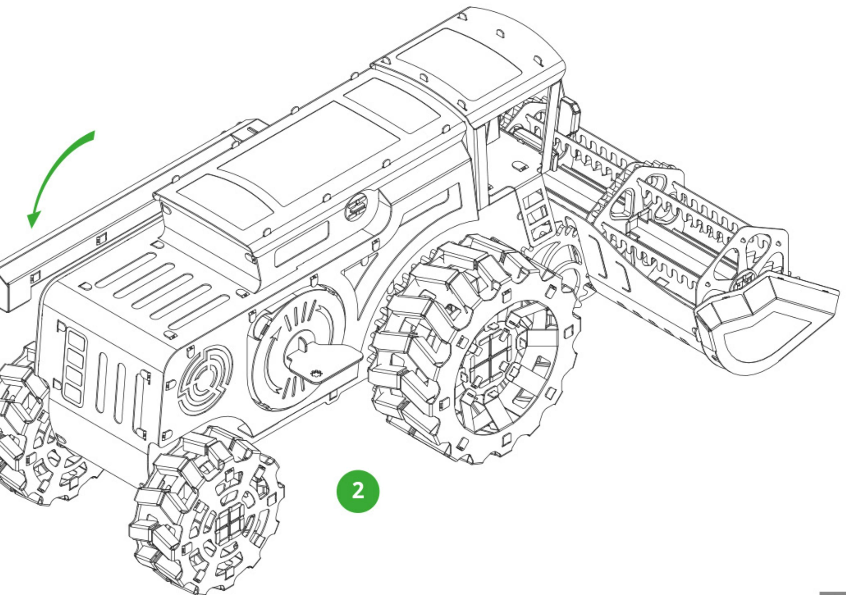
1. To prepare the harvester, raise the unloading auger, turn the mechanism clockwise with the key.
