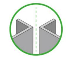
Assemble/bend parts symmetrically
