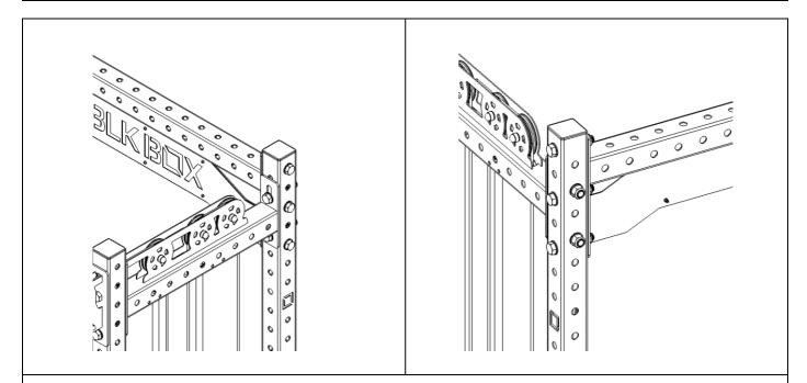
2. Insert 3x M20 Hex Head Bolts with a M20 Washer on each bolt through the first, third and fifth hole on the Upright and through the plate on the Branding Box Crossmember.
