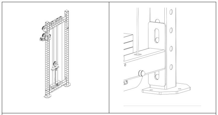
2. Line up the Pre-Assembled Frame with the Upright so that the first and third hole from the bottom line up with the slotted plate of the Bottom 0.7m Crossmember.
