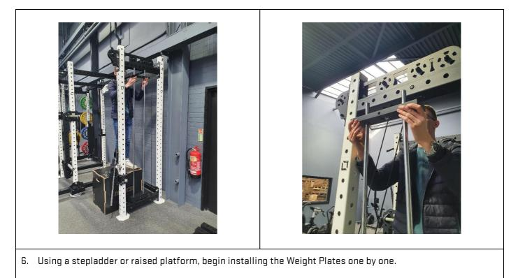
Line up the two Guide Roads with the two holes in the Weight Plates and gently slide the Weight Plate down the Guide Rod until it reaches the other Weight Plates already installed.
