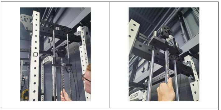
3. Tilt the Guide Rods out slightly and slide the Weight Stack Top Plate up to the top of the Guide Rods. Continue until the Weight Stack Top Plate is clear of the guide rods.
