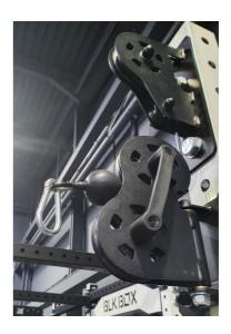
14. Once the Weight Stack is fully installed, adjust the tension in the nylon cable until the cable is slightly taught without it lifting the Weight Stack Top Plate whenever the Magnetic Selector Pin is removed.
