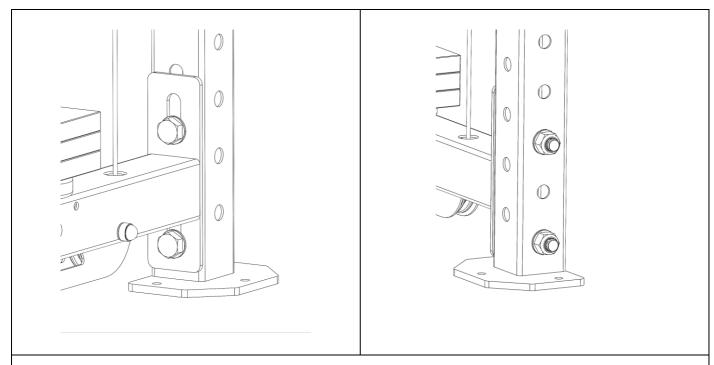
3. Insert an M20 Hex Head Bolt and M20 washer through the plate and upright. Secure on the opposite side of the upright with another M20 Washer and M20 Nyloc Nut. Tighten using 2x 30mm Spanners.
