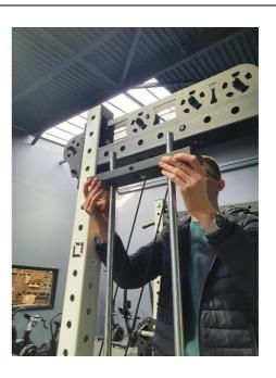
10. Using a stepladder or raised platform, begin installing the Weight Plates one by one.
