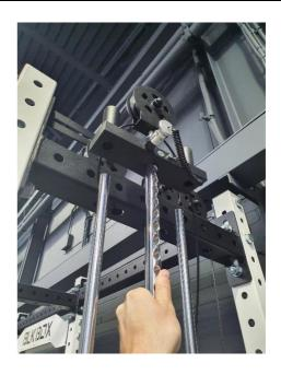
7. Tilt the Guide Rods out slightly and slide the Weight Stack Top Plate up to the top of the Guide Rods. Continue until the Weight Stack Top Plate is clear of the guide rods.
