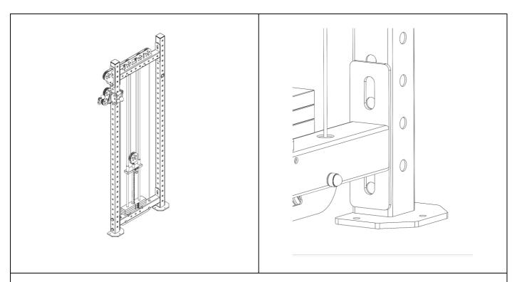
2. Line up the Pre-Assembled Frame with the Upright so that the first and third hole from the bottom line up with the slotted plate of the Bottom 0.7m Crossmember.
