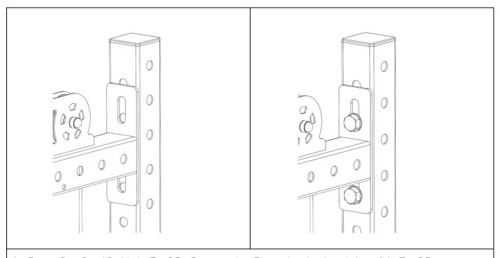
4. Repeat Step 2 and 3 with the Top 0.7m Crossmember. Ensure that the slotted plate of the Top 0.7m Crossmember lines up with the second and fourth hole from the top on the Upright.
