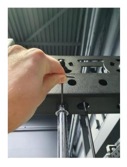
13. Reinstall the Guide Rod Locks by sliding the Guide Rod Locks on to the Guide Rods.
