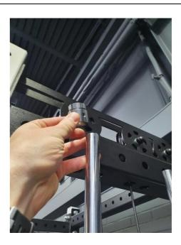
6. Start by removing the Guide Rod Locks using a 3mm Allen Key (NOT INCLUDED).
