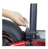
Ensure that the folding buckle is securely locked, which is a prerequisite for safe driving
