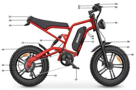
01:E-Bike display 02:Handle 03:Gear lever 04:Brake 05:Headlights 06:Front fender 07:Front wheel 08:Front fork 09:ON/OFF switch 10:Charging port 11:Battery box 12:Pedal 13:Rear derailleur guard 14:Rear Derailleur 15:Motor16:Rear wheel17:Rear fender18:Rear shock absorber19:License plate frame20:Tail lights21:Saddle
