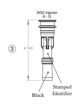
V3010-2X injectors and the V3010-2-15 Adapter include a V3283 O-RING 117 and a V3284 O-RING 114. The V3010-2-15 Adapter allows the 2" valve to be used on smaller tank sizes. The V3010-2-15 adapter can be used with any V3010-15X injector. The V3010-15X injector includes one V3416 O-RING 012 (lower) and one V3171 O-RING 013 (upper).
