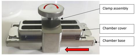
12. Hand-tighten the clamp clockwise **firmly** onto the chamber. **Only tighten, do not turn to loosen at all until hyb is complete or bubbles may be introduced and there is risk of sample leakage.**
