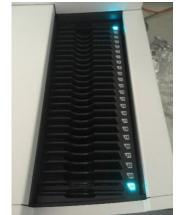
Note: Do not load empty slide holders (i.e., without slides) into the SureScan scanner!
