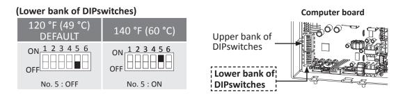
**NOTE:** Only change the switches with dark squares. The dark squares indicate the direction the DIPswitches should be set to.
