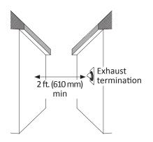
Exhaust and/or direct-vent sidewall terminations should be at least 2 ft. (610mm) away from an opposite surface/wall. Do not place the termination directly in front of an opening into a building.
