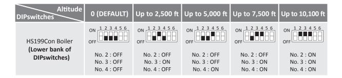
**NOTE:** The dark squares indicate the direction the DIPswitches should be set to.
