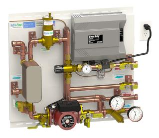
The Hydro Smart Combi Panel integrates with a wide variety of boilers and delivers "Priority" potable heated water with no storage tank and hydronic space heating in a small reliable package.
