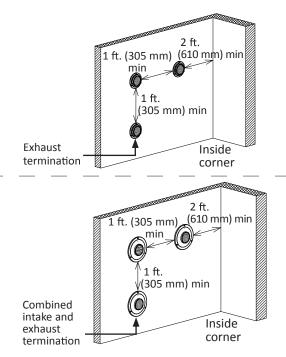
For multiple sidewall exhaust terminations (e.g. Multi-unit Systems), an exhaust termination must be at least 1 ft. (305mm) away from another exhaust termination. An exhaust termination must also be at least 2 ft. (610mm) away from an inside corner. (If the adjacent wall is less than 2 ft. (610mm) of length, the minimum required distance away from the inside corner will be equal to the length of that adjacent wall.)
