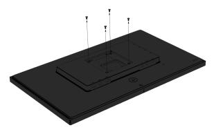
1. Remove the four mounting screws from the back of the monitor.
