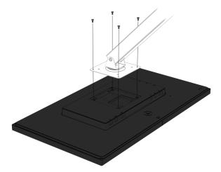
2. Align the screw holes on your mounting device with the four VESA screw holes in the back of the monitor, then insert and tighten the four mounting screws through the mounting device and into the monitor.
