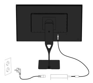
Connect the power cord to the AC adapter and plug the other end into a grounded AC outlet. Then connect the adapter to the DC power connector on the rear of the monitor.
