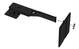
2. Slide the stand's base into the bottom of the stand arm, and then tighten the screw on the underside of the base.
