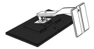
3. Insert the top of the stand into the back of the monitor cabinet at an angle, then press down. The stand will click into place.
