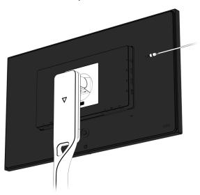
• Connect the 3.5mm audio jack plug to the audio port on the rear of the monitor to make use of your speakers, headphones, or other audio device.
