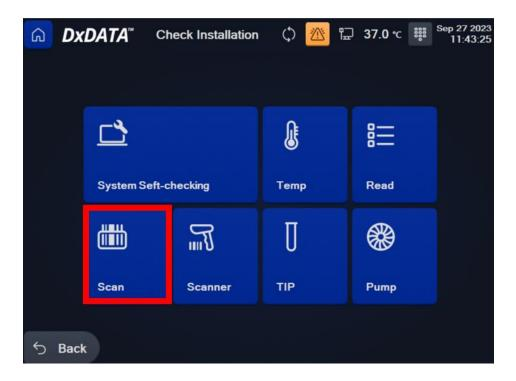
Insert 8 reagent cartridges and click "Run". System will perform internal scanner test.
