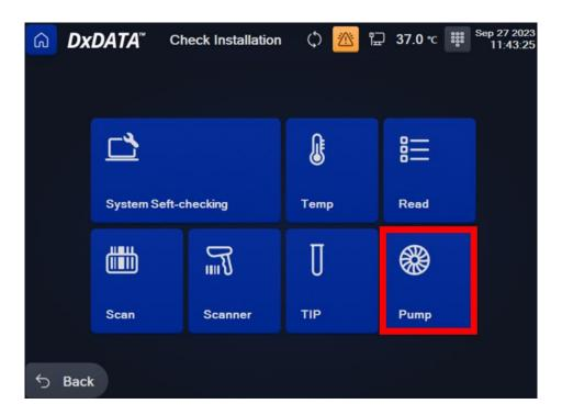
Insert 8 reagent cartridges and click "Run". System will perform air tightness test.
