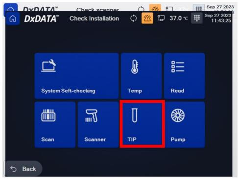
Click on "Tip" button for the pipette tips air tightness test.
