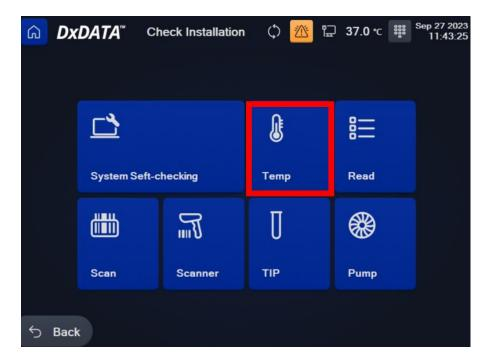
Set the number of reading times and click "Run". System will perform temperature test.
