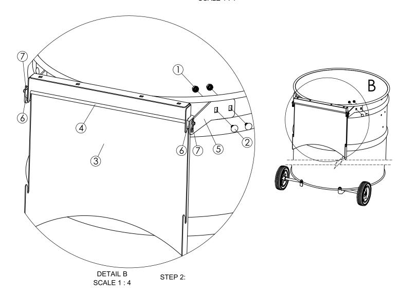
ASSEMBLE THE SHELF COMPONENTS TO THE ASSEMBLED SHELF BRACKET AS SHOWN IN DETAIL B, FOR PROPER SPACING. PLACE THE UNASSEMBLED SHELF BRACKET (ITEM 5) TIGHT UNDER THE BARREL RIM. MARK & DRILL (2) HOLES IN THE MIDDLE OF THE SLOTS. ASSEMBLE THE BRACKET TO THE DRUM, USING THE 7/16" WRENCH WITH (2) 1/4-20 CARRIAGE BOLTS (ITEM 2) & (2) 1/4-20 SEMS NUTS (ITEM 1)
