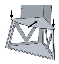
Step 5. Attach the Hearth Floor by sliding it into the slots at the bottom of the chimney. Ensure that the tabs at the corners of the Back Panels are fully engaged with the slots of the Hearth Floor.
