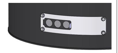
WHILE BENDING THE (3) PIECES AROUND THE DRUM, INSTALL THE OTHER (2) SELF-DRILLING SCREWS. SLIDE OPEN THE DOOR AND EQUALLY LAYOUT AND DRILL (3) 1" DIA. HOLES, ON DRUM.
