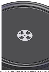
LAY EXHAUST VENT ON TOP OF LID IN LOCATION FOR MOUNTING. MARK THE CENTER HOLE AND THE (4) OTHER OPENINGS.
