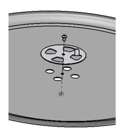
DRILL 5/16" HOLE FOR THE CENTER PIVOT HOLE.
