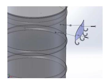
MOUNT THE HOOKS WITH THE SPACERS AND THE CARRIAGE BOLTS TO THE DRUM.
