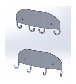
WITH ADJUSTABLE WRENCH OR PLIERS, TWIST THE (4) HOOKS OUT APPROXIMATELY 90 DEGREES.
