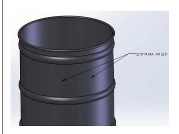
LAYOUT, MARK, AND DRILL (2) 5/16" DIA. HOLES APPROXIMATELY 8" DOWN FROM DRUM TOP LIP.
