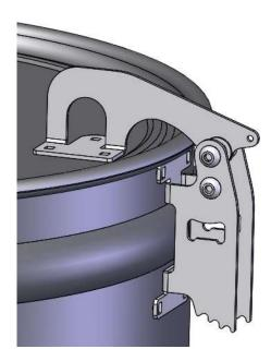
PLACE HINGE TIGHT AGAINST LID AND DRUM AND MARK (7) MOUNTING HOLES. REMOVE HINGE AND DRILL 5/16" DIA. HOLES.
