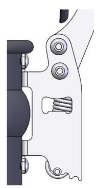
THERE ARE 3 NOTCHES ON DRUM BRACKET FOR SPRING ADJUSTMENT. MOVING THE SPRING PIN INTO THE NOTCHES FARTHER FROM THE DRUM INCREASES THE SPRING FORCE. ALWAYS ADJUST THE SPRING PIN WITH THE LID IN FULL OPEN POSITION.
