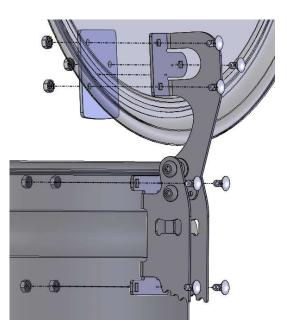
ASSEMBLE LID FIRST WITH (3) CARRIAGE BOLTS, STIFFENER PLATE AND (3) LOCK WASHER NUTS THEN MOUNT HINGE TO DRUM WITH (4) BOLTS AND NUTS.
