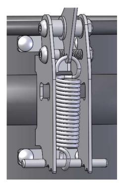
ASSEMBLE SPRING LOOP THRU HOLE ON LID BRACKET AND OPEN LID. WITH THE LID OPEN RUN SPRING PIN THRU BOTTOM LOOP OF SPRING AND PULL DOWN ON PIN AND PLACE INTO NOTHCHES OF DRUM BRACKET.
