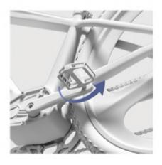
For pedal installation, please rotate and tighten with a tool. Both sides of the pedal are in the front direction.
