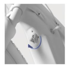
There is a key hole on the left side of frame, put the key into it and then turn about 180 degrees in clockwise, and push the active button to take out the battery case.
