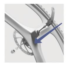
2 Loosen the nut and put the front wheel in the middle of the fork.
