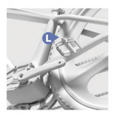
Before installation, you should observe positions of the pedal (the bottom shows the general position) L corresponds to the left as Figure (3), and R corresponds to the right (1).
