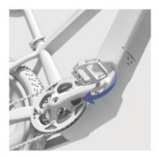
The pedal may tilt and slide during installation but it cannot be tried hard. It is necessary to find the correct position and the installation can be done easily.
