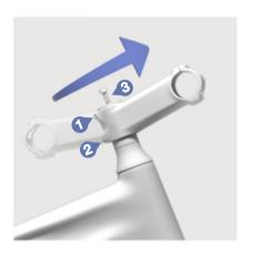
Loosen the first and second screws and rotate
