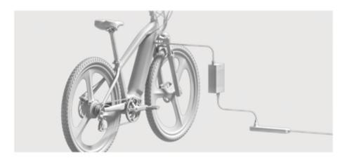
② When charging status, there is an indicator light on charger. Red color means charging, if changes to green color, it means full charge.
