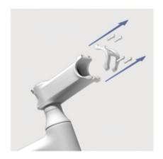
2 The top four screws are knocked down and the lid is removed.
