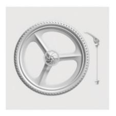
• Install the quick release parts in turn to the front wheel.
