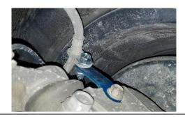
12. For 2018 and newer Crosstreks and 2019 and newer Foresters, you will need the included sway bar drop bracket. When installing this drop bracket, be sure to install it so the threaded holes are towards the front of the car in relation to the through-holes as shown. You will use the factory nuts to mount the drop spacer to the chassis and then 4 of the 20mm long M8 bolts to mount the sway bar to the spacer
