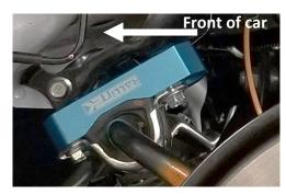
13. Reinstall the lower control arms to the subframe. This kit will get the rear alignment close to factory specifications but for proper handling characteristics and maximum tire life, we highly recommend an alignment after installation.
