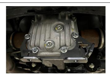
4. Slide the differential skid plate over the factory front differential support studs.
