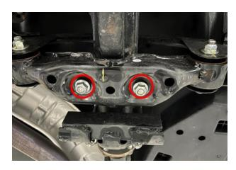
3. Install the RalliTEK differential skid plate mounting bracket onto the diff cover using supplied bolts. Thread these on hand tight for now.
