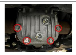
2. Locate and remove the two nuts on the front differential mounting bracket.
