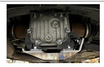
Finally tighten the bolts securing the differential skid plate mounting bracket to the differential cover to 21 ft/lbs. Then tighten the nuts on the front differential mount to 41 ft/lbs.
