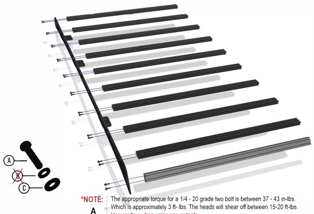
Which is approximately 3 ft- lbs. The heads will shear off between 15-20 ft-lbs. Use caution when using power tools.
