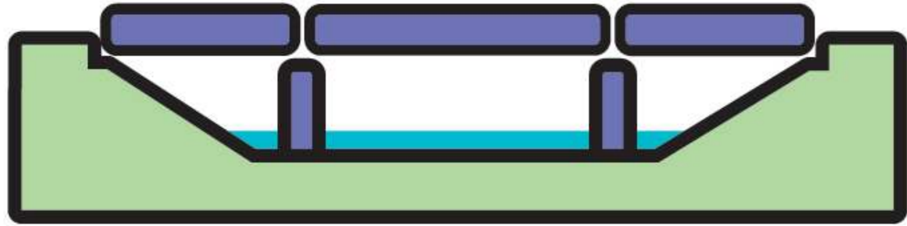
Beam Bridges go straight across.
