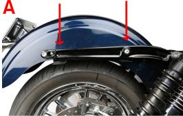
1) Locate the supplied metal L shaped anchor brackets that are listed for your bike.
