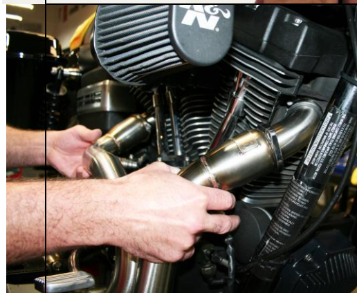
Anti-seize 02 and exhaust stud threads
