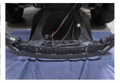
2) Measure and space the bolts along bumper, then add washer and nut and tighten
