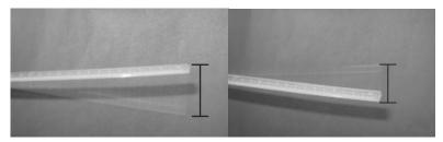
Because most of the ruler is hanging off the table, the free end can make big vibrations. The part of the ruler touching the table vibrates against the table top with a certain frequency (a certain number of times per second), and those vibrations are detected by your ears.
