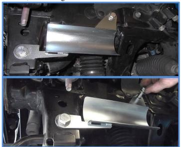
11. Reinstall skid plate using the factory hardware.
