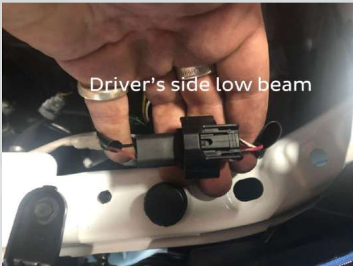
Driver's side (LH) low beam - Red to Red
