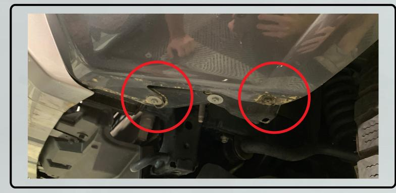
4. Remove the two 10mm screws from under the center of the bumper cover.
