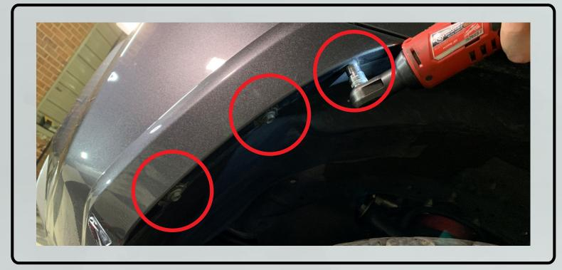
2. Remove the two (2) two-piece push clips from the corner of the top of the grille, one on each side.
