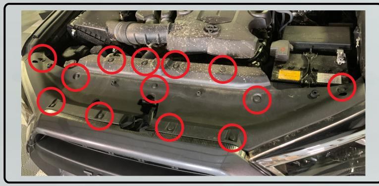
6. Remove the two push clips and 10mm bolt from the grille assembly as indicated.
