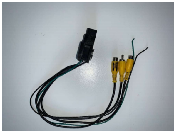
Figure 6 - Switching Relay (Two Female RCA, One Male RCA Yellow Plug)
