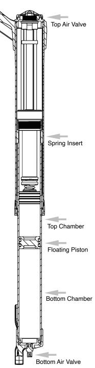
The Wren TwinAir system is a unique design that allows for fine adjustment of the air spring using only a pump. No need to disassemble the fork to insert or remove tokens.
