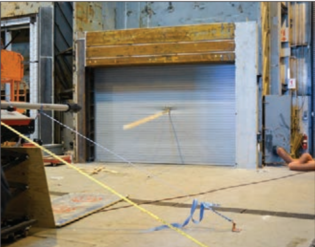
Missile impact test proves ability to withstand wind-borne debris from a hurricane or tornado.
