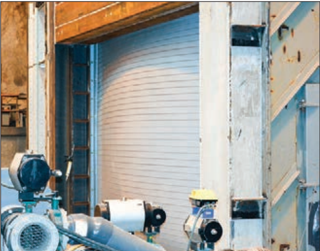
The SafeSpace 500 was subjected to both a positive and a negative 255 mph wind load.
