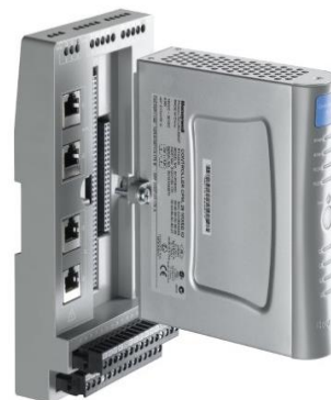
Figure 3. Positive identification on removable terminals
