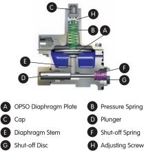
Universal Safety Shutoff Assembly (USSA) — USSA protects the downstream piping from both over- and under-pressure conditions by shutting off the gas flow at the inlet side of the regulator orifice. Both Over- and under-pressure shut-off set points are adjustable depending on spring ranges selected.
