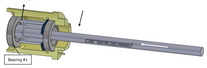
Select a drift that fits within the freehub body but meets the face of the inner diameter of the bearing, and extension tube + axel drift to enable pressing though the length of the freehub body. Use appropriate extaction cup that fits the face of the freehub body and assemble as shown.
