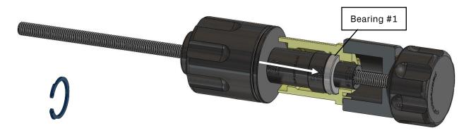
Repeat the process, this time placing the axel sleeve into the freehub body prior to pressing the second bearing into place.
