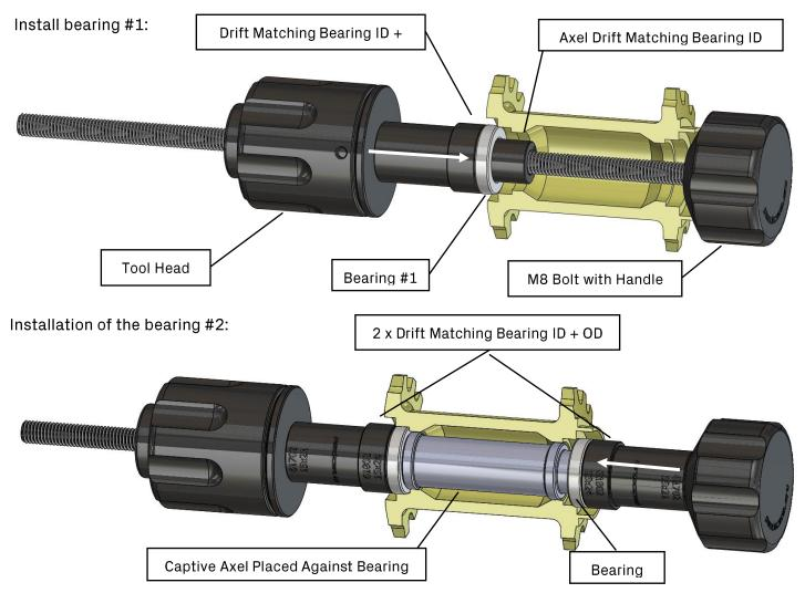
Note: Axel alignment sleeve should be used if the axel does not self align within the bearings.
