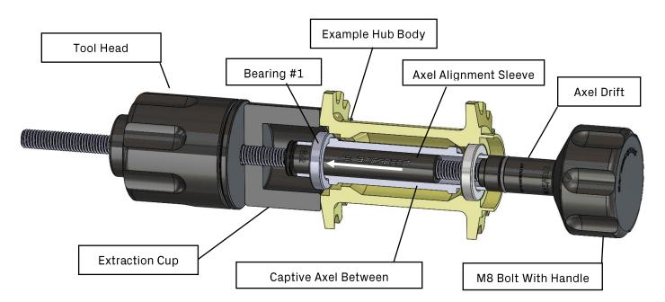
Keeping the axel inside the hub, mirror the process with the same tool arrangement and extract bearing #2.
