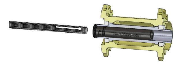
Nesting Bearing Drifts, match bearing inner diameter (small drift) and outer diameter (larger drift)
