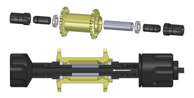
Bearing Drift matching bearing OD, with recess for over-axel design
