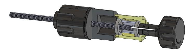
Example #3: Bearings are accessible from each freehub body face.
