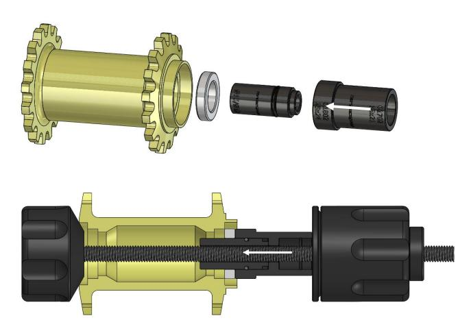
Nest Bearing Drifts used on both sides with axel ID matching bearing ID.
