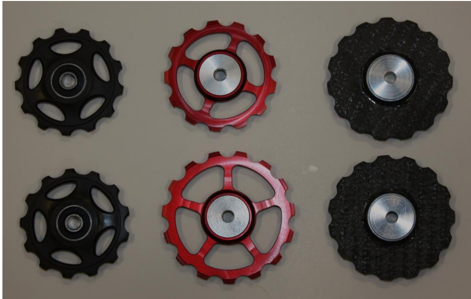
Pic 2: Oversized pulleys used for Part 2. L to R, Dura Ace 13T-13T, Berner 13T-15T, RALTech 15T-15T.
