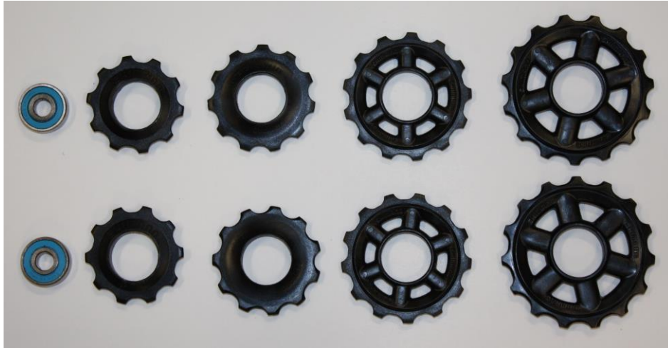
Pic 1: Shimano Acera and 105 plastic wheels with inner diameters identically milled to accept the two TACX ceramic bearings. L to R: TACX bearings, 10T, 11T, 13T, 15T.
