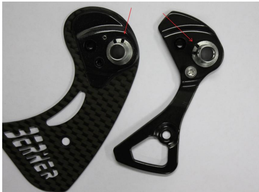
Pic 3: Red arrows indicate the different angular attachment points of the torsion spring to the cage.
