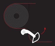
STEP 3: With the chain now cut to length it is important to test the clearance of the OSPW X System when the rear derailleur is set in the largest cog on the cassette. Just as the arrow indicates the cage should be able to rotate counter clockwise. It is important that there is some clearance between the upper pulley wheel of the OSPW X System and the largest cog on the cassette. If you find the clearance is not enough, adjust the B-tension accordingly.
