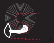
STEP 1: Place the chain on the smallest cog on the cassette. To find the correct chain length, pull the two chain ends together, just as you would when needing to cut a chain to length. The lower part of the cage should start to move downwards, away from the cassette, as referenced in the second image.
