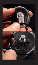
8. Place the factory alloy washer, spring and plastic cover onto the face of the OSPW X cage. Make sure that the plastic dust cover is facing the same way on the OSPW X cage as on the Shimano assembly. The flat face should sit against the OSPW X cage.
