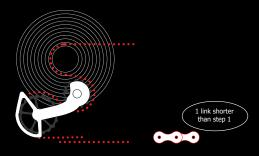
STEP 2: When tension is applied on the chain and the OSPW System appears to be aligned as the diagram above, cut the chain 1 full link (inner + outer link combination) shorter to ensure adequate chain tension is present in all gears (small chain ring/smallest cog allowed on the cassette).
