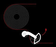
STEP 3: With the chain now cut to length it is important to test the clearance of the OSPW Aero System when the rear derailleur is set in the largest cog on the cassette. Just as the arrow indicates the cage should be able to rotate counter clockwise. It is important that there is some clearance between the upper pulley wheel of the OSPW Aero System and the largest cog on the cassette. If you find the clearance is not enough, adjust the B-tension accordingly.
