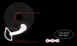
STEP 2: When tension is applied on the chain and the OSPW Aero System appears to be aligned as the diagram above, the chain needs to be cut (1 link shorter than step 1) and connected by the required amount of links in order to achieve sufficient tension in this gear combination (always the small cog on the cassette).
