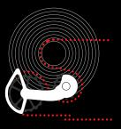
STEP 1: Place the chain on the smallest cog on the cassette. To find the correct chain length, pull the two chain ends together, just as you would when needing to cut a chain to length. The lower part of the cage should start to move downwards, away from the cassette, as referenced in the second image.
