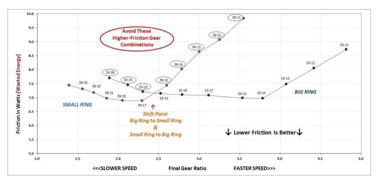
In graphs 1 and 2, the bottom axes are not to scale as the bar graph is used to provide an easy-to-read visual representation of the proper shift pattern and specific big-to-small ring and small-to-big ring shift points. Graph 3, above, shows the gear combinations on a correctly-scaled bottom axis of effective final gear ratio. The light blue data points represent the small ring with each of the 11 cogs. The dark blue data points represent the big ring with each of the 11 cogs.
