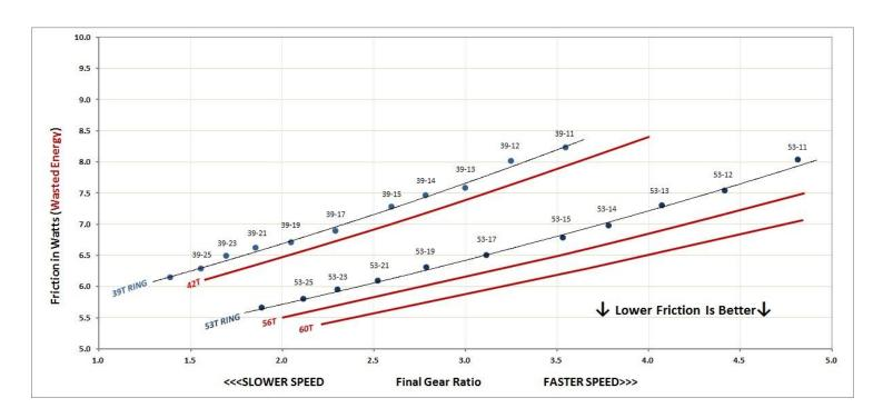
Based on the results and curves obtained with the data, it is speculated that the frictional losses of ring and cassette combinations other than 53T, 39T, 11-28T can be determined, and new shift points found for the new combinations. In order to determine frictional losses of different combinations, the effects of different rings must be analyzed first, and the effect of different cassettes can then be analyzed.
