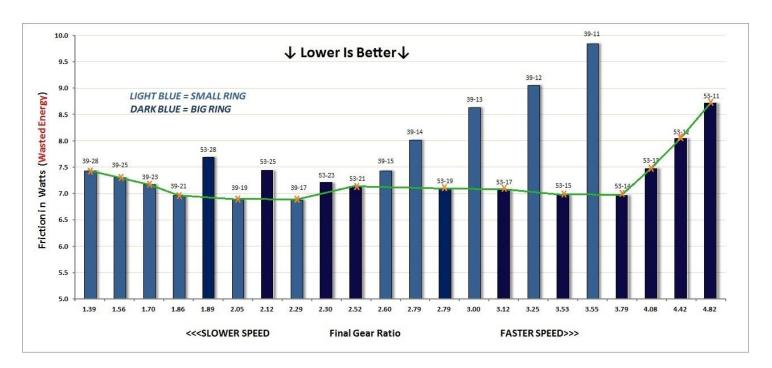
Graph 2 shows *all* 22 ring-cog combinations including the 8 higher-friction ring-cog combinations which were not included in Graph 1. The green line represents the shift pattern, and connects the most efficient gear combinations when increasing or decreasing speed.
