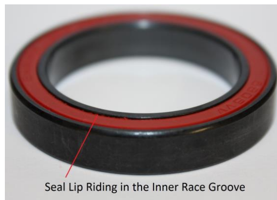
Photo 4: The Enduro Bearing with seals installed, showing the light contact design, with the seal lip contacting the inner race.
