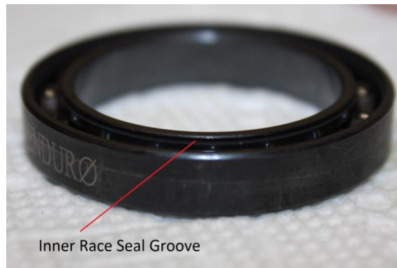
Photo 3: The Enduro Bearing with seals removed, showing the light-contact design, with the Inner Race Seal Groove visible.
