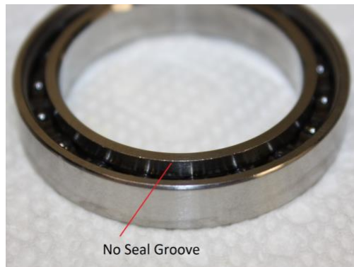
Photo 1: The Gold Race Bearing with seals removed, showing the non-contact design, with no seal groove on the inner race
