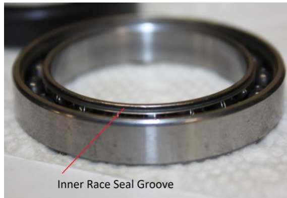
Photo 5: The CeramicSpeed Bearing with seals removed, showing the light-contact design, with the Inner Race Seal Groove visible.
