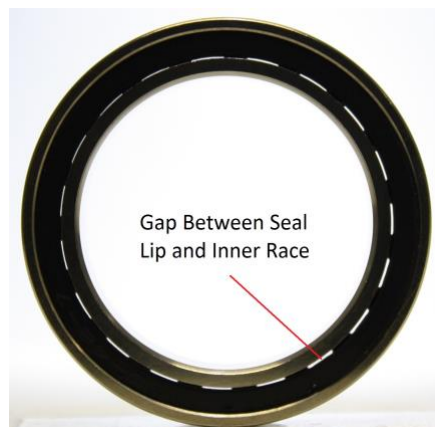
Photo 2: The Gold Race Bearing with front seal installed, showing the non-contact design, with the gap between the seal lip and inner race visible.
