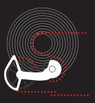
STEP 1: Place the chain on the smallest cog on the cassette and the small front chain ring. To find the correct chain length, pull the two chain ends together, just as you would when needing to cut a chain to length. The lower part of the cage should start to move downwards, away from the cassette, as referenced in the second image.
