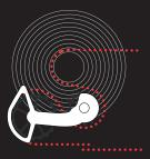
STEP 1: Place the chain around the front chain ring, smallest cog, and through the derailleur. To find the correct chain length, pull the two chain ends together, just as you would when needing to cut a chain to length. The lower part of the cage should start to move downwards, away from the cassette, as referenced in the second image.
