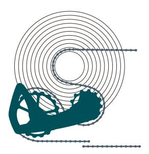
**STEP 1:** Place the chain on the smallest cog on the cassette and the small front chain ring. To find the correct chain length, pull the two chain ends together, just as you would when needing to cut a chain to length. The lower part of the cage should start to move downwards, away from the cassette, as referenced in the second image.
