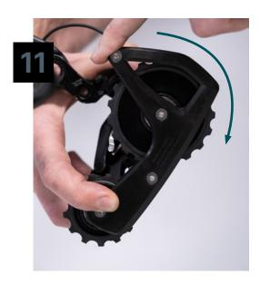
Hold the OSPW RS cage against the derailleur body and rotate counter-clockwise (first up and then to the back of the bike and downward) until you feel the ramped stop tower click past the stop point on the derailleur.
