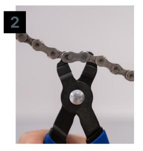
Remove the chain with a proper chain tool. Upon completion of installing the OSPW. System you will need to use a new, longer chain.
