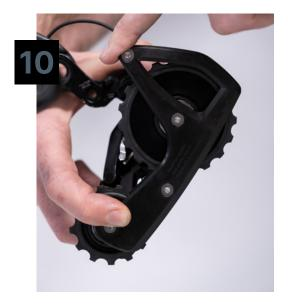
Rotate the derailleur body back, align the mounting post of the OSPW RS System to the back of the derailleur body with the cage pointing to the front of the bike. Align the tension spring and plastic spacer with the slot on the derailleur body and insert until the cage is flush to the derailleur. Ensure the OSPW cage rotates smoothly and the spring is properly secured.
