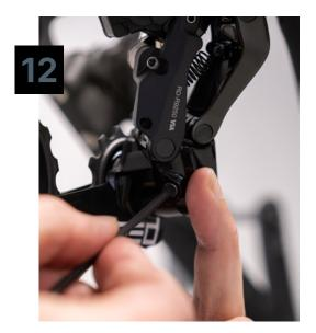
Secure the cage by reinstalling the original black T10 screw (removed at step 3). Installation torque is 1Nm. Your new OSPW System is now installed.
