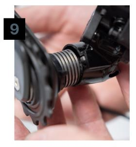
Select the spring tension hole second from 'L' (second lowest tension) and insert the hooked end of the spring completely. This may need to be pressed firmly. The plastic spacer will rest freely on the spring until aligned at the back of the derailleur body.
