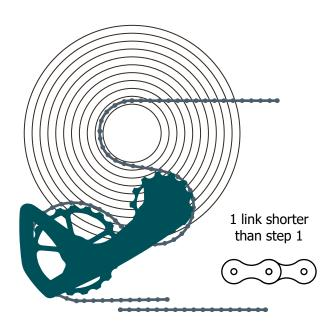
**STEP 2:** When tension is applied on the chain and the OSPW RS System appears to be aligned as the diagram above, the chain needs to be cut (1 link shorter than step 1) and connected by the required amount of links in order to achieve sufficient tension in this gear combination (always the small cog on the cassette).
