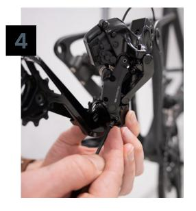
Shift the derailleur up to the cage can rotate past the body. For Ultegra 8150 or 105 7150, remove the rotation stop screw using a Philips screwdriver, and carefully allow the cage to unwind. For Dura Ace 9250, pull the cage by hand away from the derailleur body until the stop tower is free and carefully allow the pulley cage spring to unwind, releasing the spring tension. Your derailleur cage will appear to be upside down.
