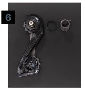
Remove the spring and plastic spacer from the Shimano cage. The end of the spring is hooked to lock into the pulley cage. Keep these aside as you will reuse these for the installation of the OSPW RS System on Ultegra 8150 or 105 7150. You do not need the plastic spacer for the Dura Ace 9250 as you will use the thicker spacer supplied with the OSPW RS System.
