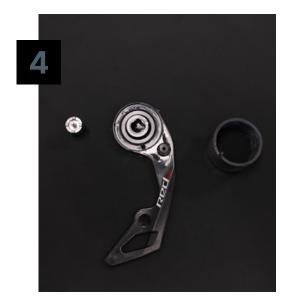
Remove the main center nut and the stock cage. There will be a small amount of spring tension on the cage due to the clutch. Set aside the spring and center nut for reuse.
