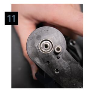
Mount the cage on the center screw and thread the center mounting nut into place using the provided 4 prong tool. Finger tighten the nut until firm, and then unthread 360 degrees (1 full turn). The D-interface will not be aligned at this point.
