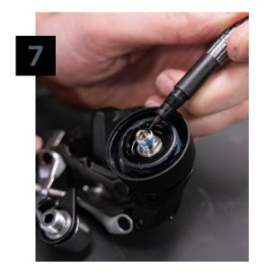
Mark the center screw end with a pen to identify the flat surface of the D on the bottom of the center screw (A).
