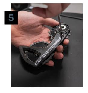
Unbox the CeramicSpeed OSPW RS system and remove the rotation stop screw (to be reinstalled once the cage is mounted). Dissasemble the OSPW RS System by removing all 4 bolts from the back of the OSPW RS System. Set aside the 4 bolts, back cage plate, and both pulley wheels.
