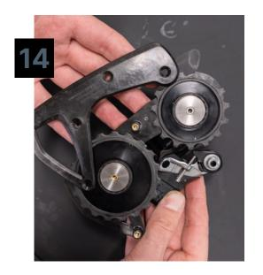
Install the 15 tooth pulley on the upper post and the 19 tooth pulley on the lower post of the OSPW RS cage. Ensure the etching on the pulleys face outwards (facing the cage plate with the logo). Align the back cage plate and use a 2.5mm allen key to install both pulley screws to a torque of 1Nm, and a 2.0mm allen key for the center and lower tower screws to a torque of 0.3Nm
