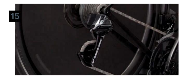
Install the derailleur onto the bike. Shift down to the bottom (smallest cog) and install the rear wheel. Measure a new chain following the guide below and check the upper and lower stop screws as well at the b-limit adjustment following the factory SRAM guidelines; 14mm for a 26T cog, 10mm for a 28t cog, 5mm for a 33T cog.
