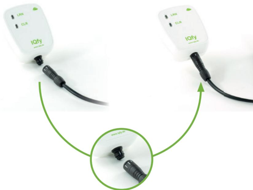
**Important notice:** This is a **connector**, please do not twist the plug onto the connector. You will find a white line on both the radio receiver and the adapter cable you will find a white line as a mark - these must fit over each other.
