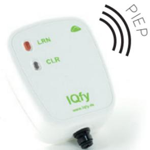
2a Connect the motion detector directly to the the NAVI radio receiver for targeted Alarm triggering via the nurse call system if the IQcare bed escape system is already connected (**working current mode**).
