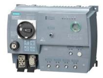
SIRIUS motor starter M200D AS-i communication: AS-Interface direct-on-line starter basic mechanical switching AC-3, 0.75 kW/400 V 0.15 A...2.00 A electronic overload protection thermistor: thermoclick / PTC without brake contact 2 DI AS-i + 2 DI / 1 DO on device Han Q4/2 - Han Q8/0 with manual on-site operation and keyswitch
