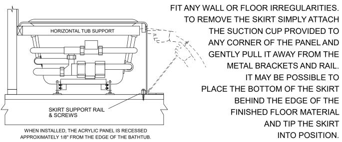
IT IS THE INSTALLER'S OBLIGATION TO INSURE THAT THE SKIRT FITS PROPERLY AND IS NOT UNDER STRAIN OR TWISTED. THE SKIRT CAN BE TRIMMED, BUT CARE SHOULD BE TAKEN WHEN CUTTING IT. CALL WATERTECH IF YOU NEED HELP OR SUGGESTIONS. 1-800-795-7480
